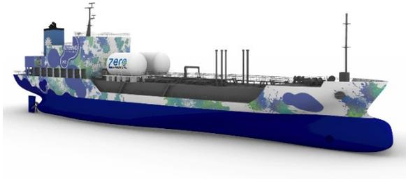
The image of this ship with a concept of arranging the hydrogen fueled engine as power generator in engine room for electric propulsion
